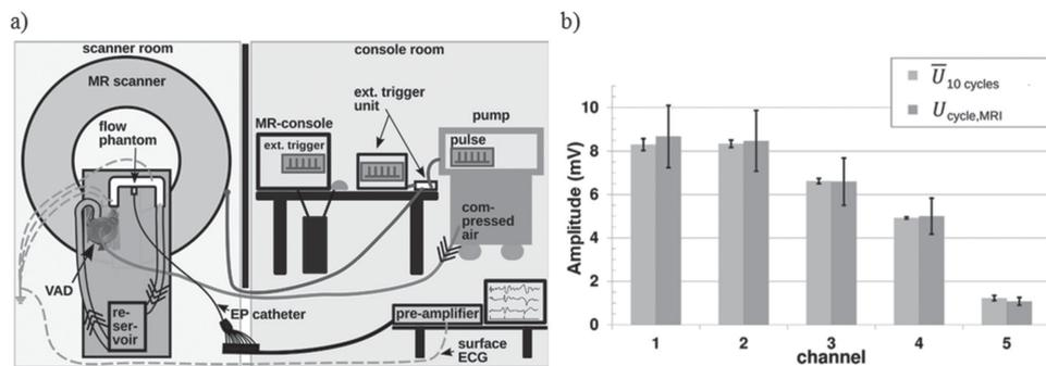
**Figure 4.** Development of an MHD surrogate model for the validation of induced VMHD as a blood flow potential. a) Experimental design for the recording of induced VMHD using an EP catheter located within a flow phantom. b) Comparison of MRI flow derived VMHD ( $U_{10 \text{ cycles, MRI}}$ ) and measured VMHD ( $U_{10 \text{ cycles}}$ ) in the flow phantom over ten cycles, illustrating flow dependence.
