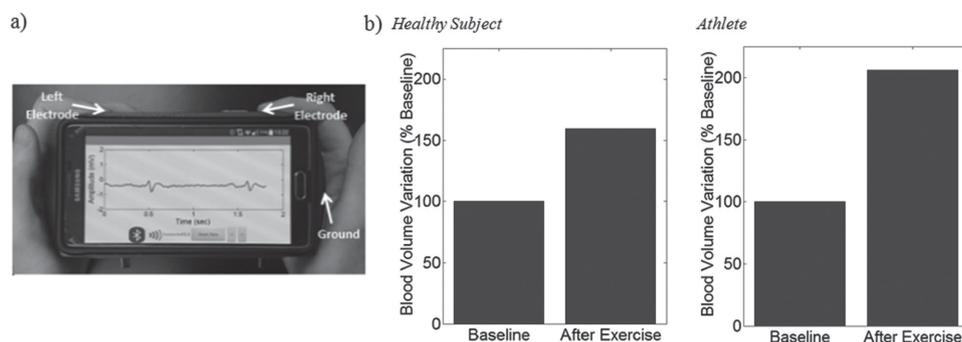
**Figure 7.** Development of a portable device for quantifying induced MHD voltages and estimated variations in blood flow during exercise stress testing. a) Typical usage of prototype portable flow monitoring device, illustrated during ECG acquisition. b) Time-integrated SV metrics during exercise stress testing in a normal health subject (left) and in an athlete (right).
