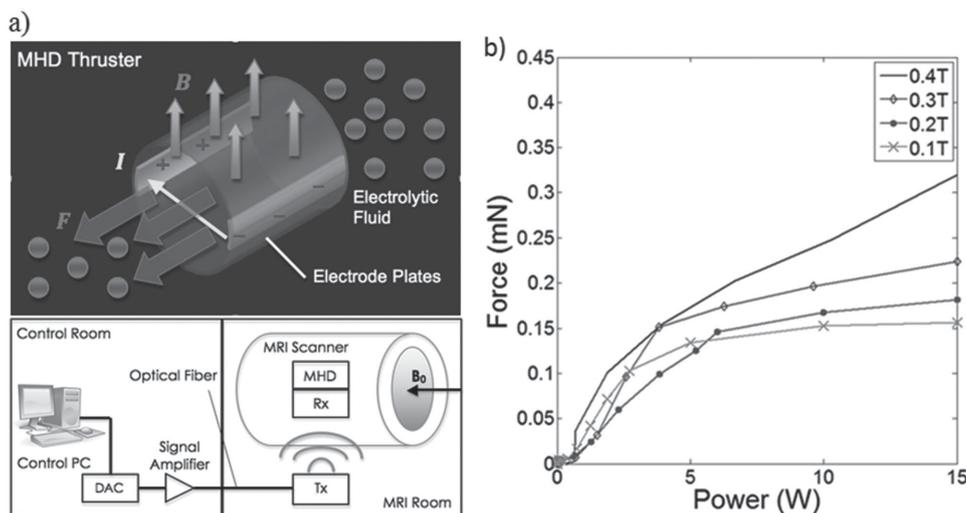
**Figure 2.** Development of an MRI-compatible magnetohydrodynamically driven endocapsule. a) Translation of the MHD effect into a source of propulsion (top), and the design of an MHD thruster for use in an MRI scanner (bottom). b) Quantification of system dynamic performance; step input response.
