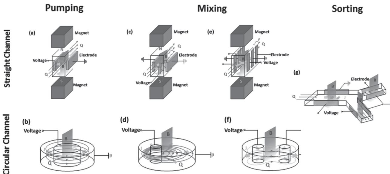
**Figure 1.** MHD based microflow manipulations: a) DC operated micropumps in a straight channel and b) a circular channel; c,e) AC operated micromixer in straight channels and d,f) circular chambers; and g) MHD micropump based sorting device. Images are reproduced from refs. [14,24,25,27,30] and [31].
