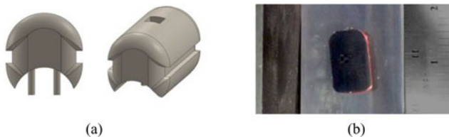
Fig. 7. Experimental design for quantification of system performance using enclosed raft design in vasculature surrogate. (a) Sealed endocapsule preliminary design: front view (left) and oblique view (right). (b) Sealed endocapsule in conduit (middle) next to magnet (left) and scale (right).
