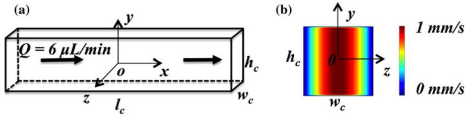
**Fig. 2** **a** Dimensions of a microchannel (listed in Table 1) with length  $l_c$ , height  $h_c$  and width  $w_c$ . A laminar flow with flow rate  $6 \mu\text{L}/\text{min}$  is introduced into the channel in positive  $x$ -direction. **b** A representative velocity distribution in the  $y$ - $z$  plane at flow rate  $6 \mu\text{L}/\text{min}$
