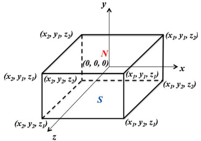
**Fig. 1** A rectangular permanent magnet located in Cartesian coordinates with its magnetization facing negative  $y$ -direction. Eight corners of the magnet are at  $(x_1, y_1, z_1)$ ,  $(x_1, y_1, z_2)$ ,  $(x_1, y_2, z_1)$ ,  $(x_1, y_2, z_2)$ ,  $(x_2, y_1, z_1)$ ,  $(x_2, y_1, z_2)$ ,  $(x_2, y_2, z_1)$  and  $(x_2, y_2, z_2)$
