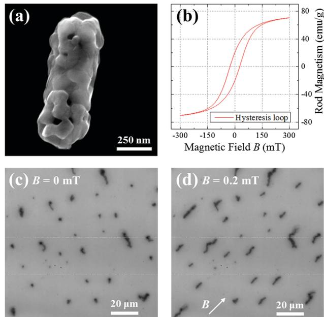
Fig. 1 (a) A representative SEM image of a single  $Fe_3O_4$  microrod. (b) The magnetic hysteresis loop of  $Fe_3O_4$  microrods. An optical microscope image of rod clusters at (c)  $B = 0 \text{ mT}$  and (d)  $B = 0.2 \text{ mT}$ . The  $B$ -field direction is indicated by a white arrow.
