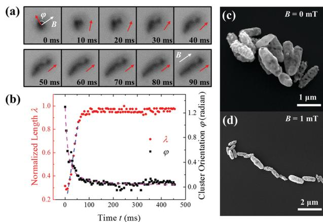
Fig. 2 (a) Representative video frames of the extension–rotation coupling motion of a FMRC with  $L_s = 9 \mu\text{m}$  at  $B = 1$  mT. (b) The plots of the normalized length  $\lambda$  (red circles) and the orientation  $\varphi$  (black squares) with respect to time  $t$ , extracted from the magnetic cluster shown in (a). The dashed curves are the fitting results. Representative SEM images of a FMRC at (c)  $B = 0$  mT, and (d)  $B = 1$  mT.
