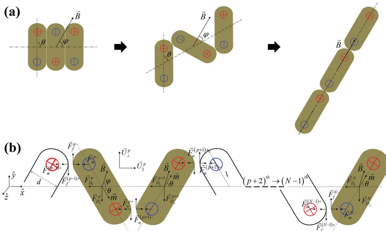
**Fig. 3** (a) The proposed dynamic process for a side-by-side chain to be extended to an end-to-end chain via a zig-zag chain model triggered by an external  $B$ -field. (b) Force and torque analysis on a pair of the  $p^{\text{th}}$  and  $(p+1)^{\text{th}}$  rods (color filled,  $1 \leq p \leq N-2$ ), and the  $N^{\text{th}}$  rod in the half chain at any time  $t$ .
