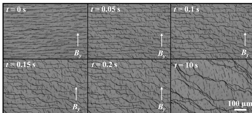
**Figure 1.** Movie clips of the morphological change of the FMRs when  $B_y$  was applied at every 0.05 s for  $C_R = 0.5 \text{ mg ml}^{-1}$ . At  $t = 0 \text{ s}$ , long chains were formed after applying  $B_x = 25 \text{ mT}$  for 150 s.
