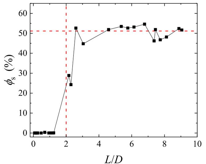
**Figure 4.** The plot of the saturation cellular fraction  $\phi_s$  versus  $L/D$  for  $B_x = 25 \text{ mT}$  and  $B_y = 5 \text{ mT}$  for different  $C_R$ . The critical condition  $L/D = 2$  and the saturation  $\phi_s$  is marked by a red dash line.
