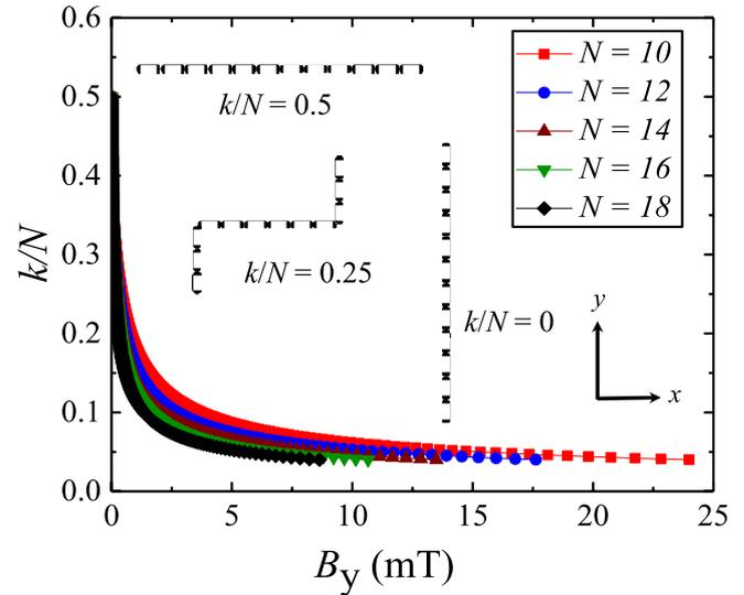
**Figure 7.** Numerical prediction of the bending length ratio  $k/N$  and the magnetic field  $B_y$  (1–25 mT) for different chain length  $N$ . The inserts show the possible chain bending configurations for  $k/N = 0$ , 0.25, and 0.5 at  $N = 12$ .
