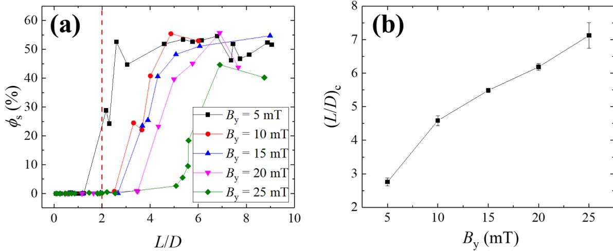
**Figure 8.** (a) The plots of the saturation cellular fraction  $\phi_s$  versus  $L/D$  under different  $B_y$ . (b) The plot of the critical  $(L/D)_c$  versus  $B_y$  for  $\phi_s = 50\%$ .
