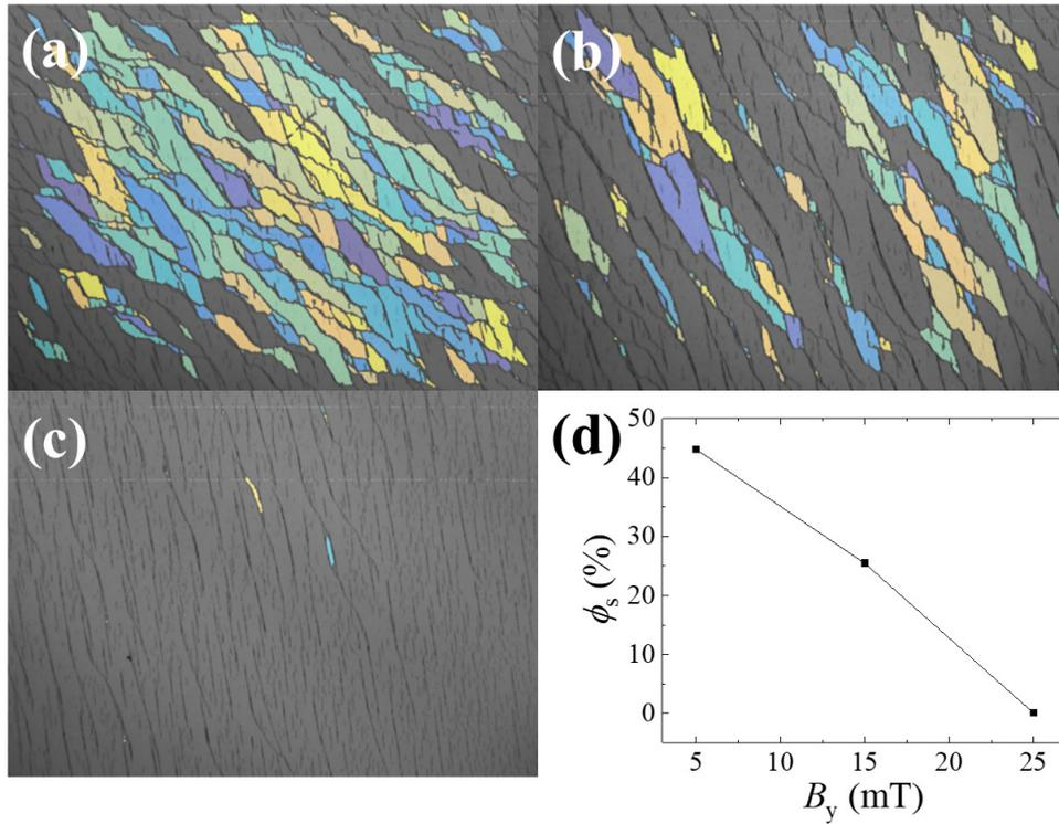
**Figure 5.** The saturation cellular structures formed at (a)  $B_y = 5$  mT, (b)  $B_y = 15$  mT and (c)  $B_y = 25$  mT, respectively, for the same initial conditions  $C_R = 0.3$  mg ml $^{-1}$ ,  $B_x = 25$  mT, and  $\Delta t = 150$  s. (d) The plot of the saturation cellular fraction  $\phi_s$  versus  $B_y$  obtained in (a)–(c).
