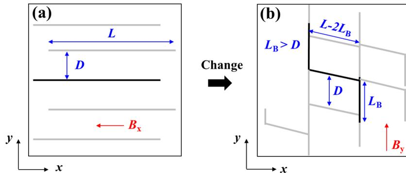
**Figure 3.** (a) The schematics of the initial chain morphology; and (b) the geometrical relations of  $L_B$  and  $D$  to form a closed loop.
